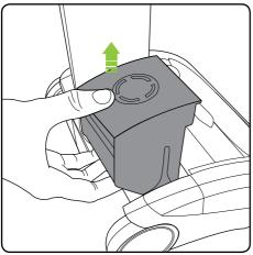
If the brush bar jams during use, the AirRam will stop and the LEDs will appear red. Before checking for a blockage, remove the battery.
