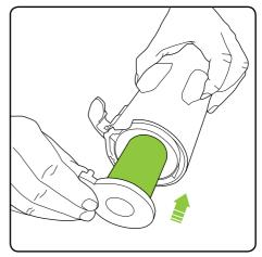
Slide the filter back into the dirt bin.
