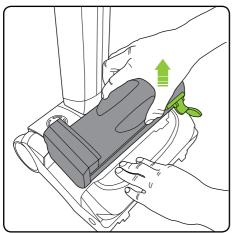
Firmly hold the AirRam with one hand and pull the dirt bin handle and lift the dirt bin our of the AirRam.
