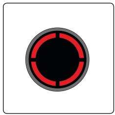
If the brush roll jams during use, the AirRam will stop working and the LED's will appear red. You will need to remove the battery first, and then remove the brush roll to clean it.
