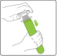
Firmly hold the filter and with the other hand grasp the separator cap. Gently pull the filter and separator cap apart. (Gently twisting and pulling will help separate the two parts.)
