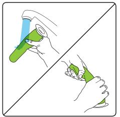
You may gently wash the filter under warm water. Do not use detergents or soaps. The filter must be completely dry before reinserting into the AirRam.
