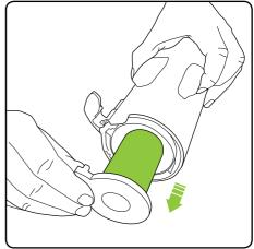
Pull the filter out of the dirt bin. Tap the dirt from the filter and tip any dirt from the filter housing. Wash the filter if necessary.
