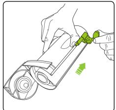
Pull the green lever back towards the bottom of the dirt bin. Close the dirt bin lid and reinsert into the AirRam.
