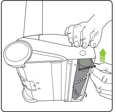
Re-insert the brush roll, starting by locating the end furthest away from the button. Then push the brush roll into the AirRam until it clicks into place.
