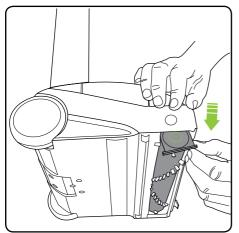
The brush roll can now be removed, starting at the button end.
