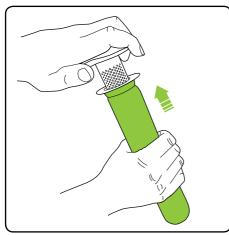
Slide the filter onto the separator.
