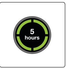
The battery can be charged from flat in 5 hours. The state of charge indicator will show 4 green lights when it is charged. It is OK to charge for 1 hour for a burst of cleaning.
